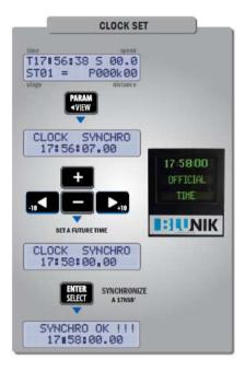
To synchronize the BLUNIK clock, enter the exact hour, minute, and second. When the reference clock displays the desired time, press **ENTER**.
