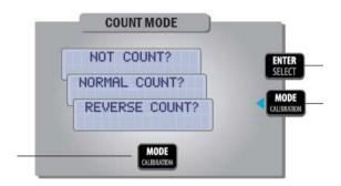
You can stop sensor readings or make it subtract meters. To do so, you must select the way in which the sensor counts kilometers by pressing the **MODE** key.
