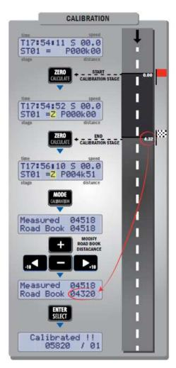
From the current screen, press the **ZERO** button at the exact point where the calibration zone begins.
