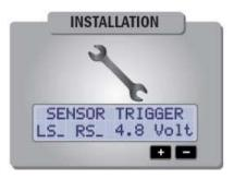
BLUNIK has compatible connections with inductive proximity sensors for 2 and 3 cables.
