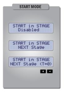
This parameter indicates the function that the **START** button executes <u>during</u> an active stage.
