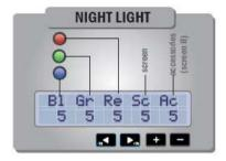
With this option you can manage the level of brightness for the three indicator lights, as well as the BLUNIK screen and the accessory screens in night mode.
