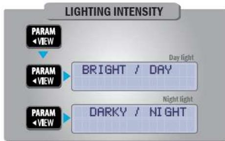
You can adjust the nighttime brightness level in advance using the night lighting parameter.
