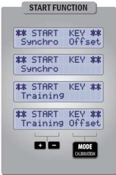
With this parameter you can define how BLUNIK will work when you press **START** to activate a specific stage.
