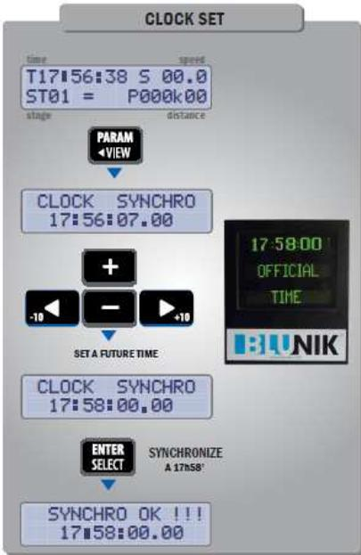
To synchronize the BLUNIK clock, enter the exact hour, minute, and second. When the reference clock displays the desired time, press **ENTER**.
