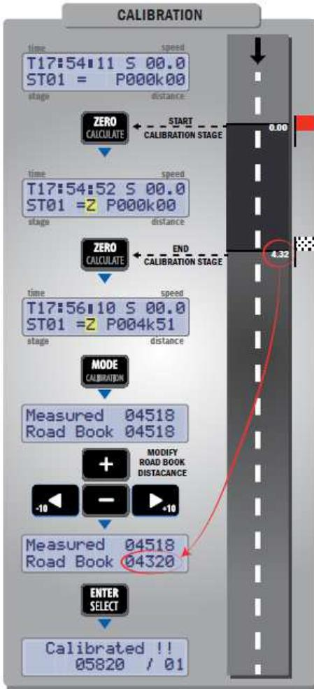
From the current screen, press the **ZERO** button at the exact point where the calibration zone begins.
