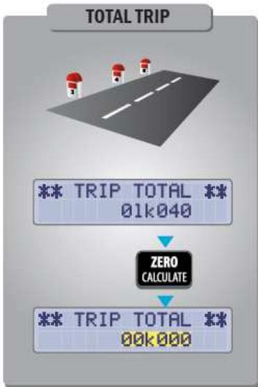
This parameter shows the total distance covered from the last setting of the parameter to zero.
