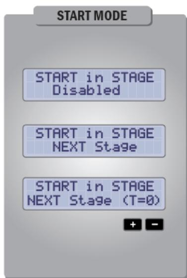
This parameter indicates the function that the **START** button executes during an active stage.
