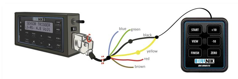
Extra Blunik II keypad for segment functions. Useful for navigators anchored to the bucket seat. Put it wherever you want.
