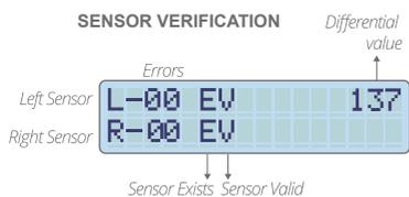
To verify the perfect functioning of the sensors we enter the Calibration screen and then press **MODE CALIBRATION**
