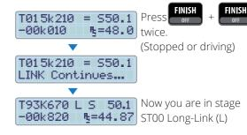
The total distance is the sum of the distance traveled in ST00 and the distance traveled in the stages ZR. (The programmed Offset distance is not added)
